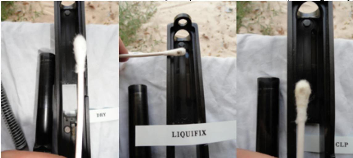
Lubed and shot 75 rounds to measure (Residual oil an Debris build up/release)
